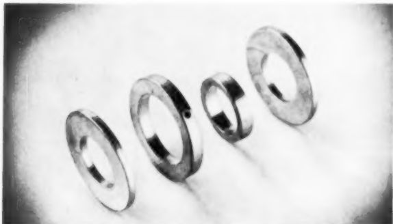
PLI-22 Preload Indicating Washers are used with the EWB-22 to induce correct preload in the bolt. They provide the most precise known method for preloading bolts during production assembly operations. They are sandwiched between close tolerance hardened steel washers.
